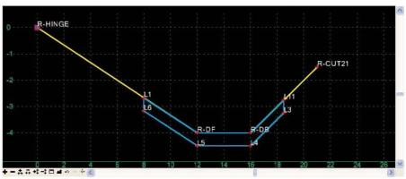
Here, the ditch has been added to a template. Notice when the template is tested, a liner is present even when the template is in fill.
